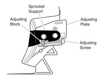
Figure 4 - Part Locations for Assembling Guide Bar
